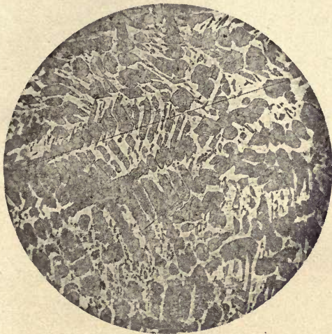
Fig. 43. × 135 Alloy 73. Cu 75·0 Annealed at 560° C. Sn 15·0 quenched. Zn 10·0.
